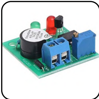
Under Voltage Alarm
