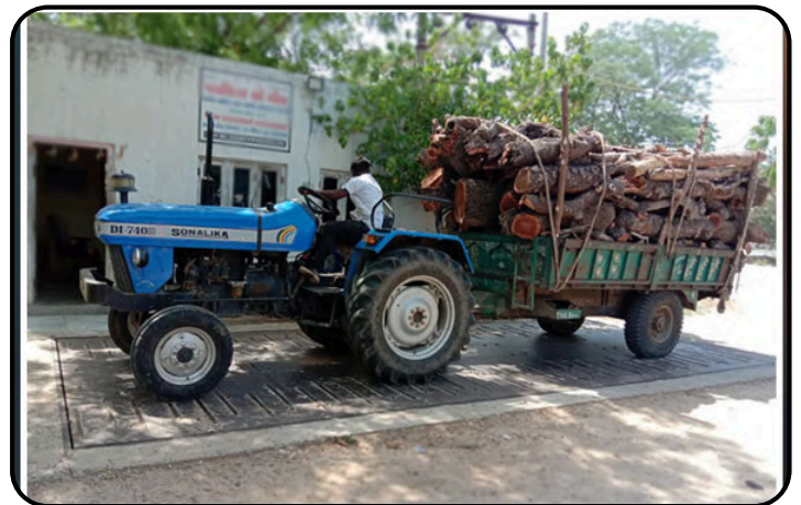
Pit Type Weighbridge
